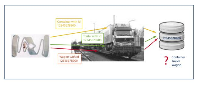
**Illustration 1:** *RFID Tag with an individual, owner specific identification stored in the data base (leads to different objects with the same identification)*
