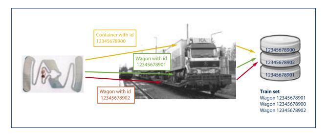
**Illustration 2:** *RFID Tag with an individual, owner specific identification stored in the data base (leads to misinterpretation of which object has been observed)*
