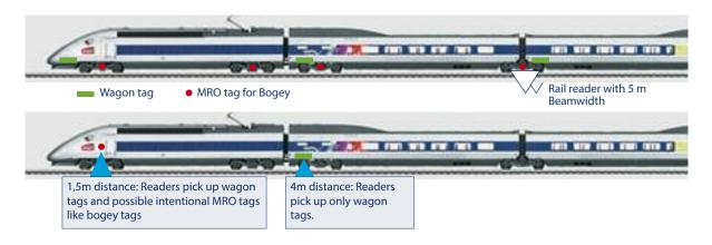
\* Current empiric tests have shown that trackside reader systems can cope with 3 visible tags on a 5 m segment of trains up to 160 km/h and with only 1 visible GIAI-96 tag on a 5 m segment of train at speeds of 200 km/h.
